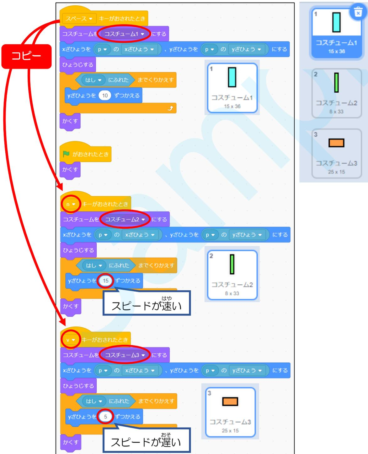
The image shows a Scratch code editor with three key events. A red arrow labeled "コピー" (Copy) points from the first event to the second. The second event has a callout "スピードが速い" (Speed is fast) pointing to the speed value "15". The third event has a callout "スピードが遅い" (Speed is slow) pointing to the speed value "5". A costume palette on the right shows three costumes: Costume 1 (15x36), Costume 2 (8x33), and Costume 3 (25x15).
